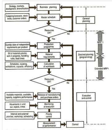
Around 1980, over-frequent changes in sales forecasts, entailing continual reajustments in production, as well as the unsuitability of the parameters fixed buy the system, led MRP (Material Requirement Planning) to evolve into a new concept: Manufacturating Resource Planning or MRP2
