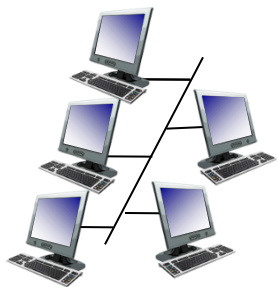
shared wire (e.g., cabled Ethernet)
